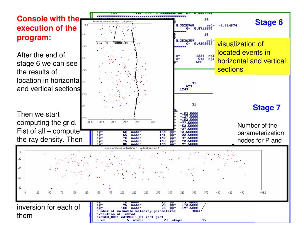
After computing the grid, we can see the distribution of nodes and ray paths in hor. and ver. sections.
