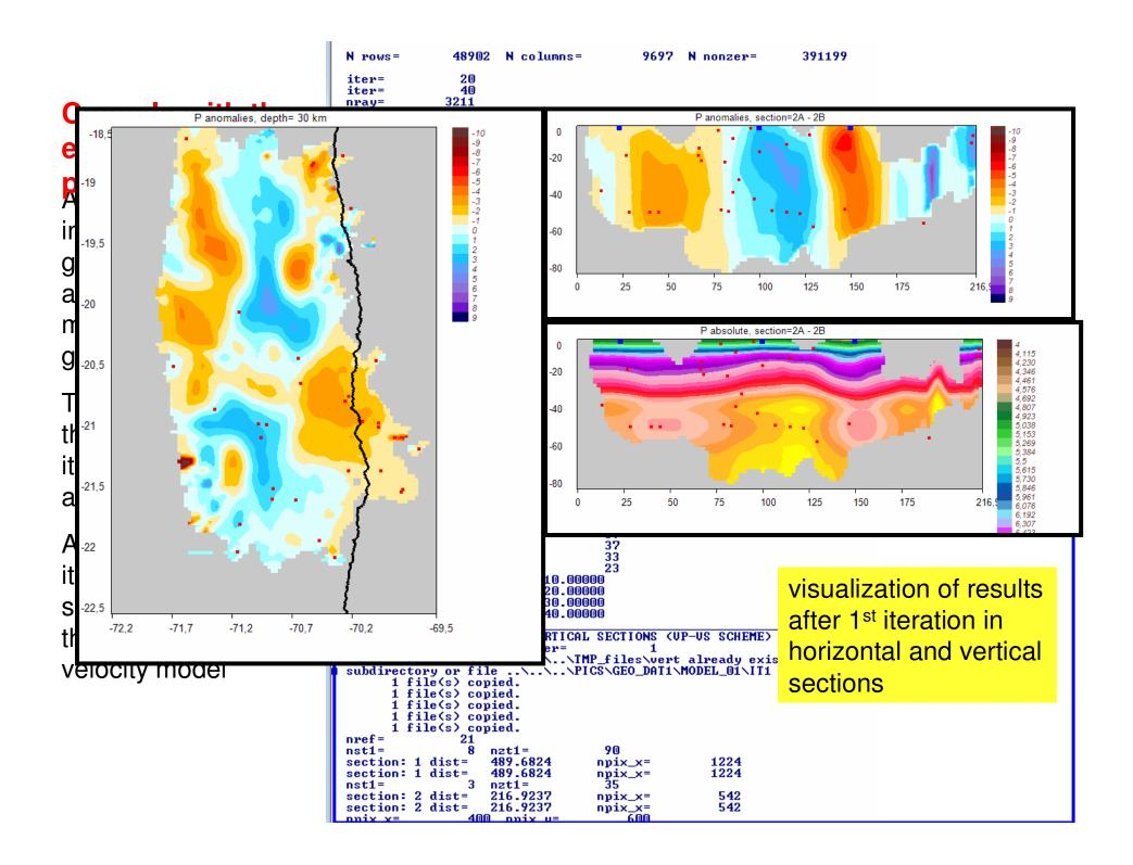
The 2<sup>nd</sup> iteration starts with source location in the updated 3D velocity model.
