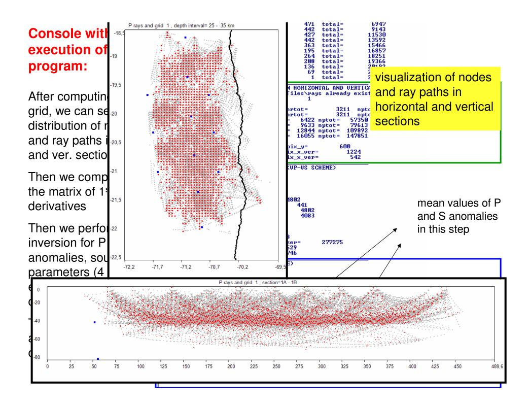
After performing inversion for all grids, we compute an average 3D model in a regular grid
